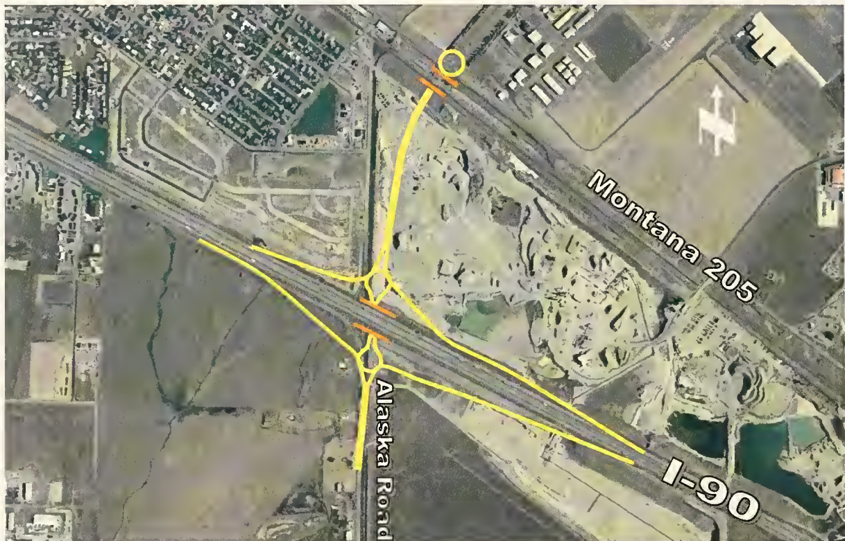
Figure 2-7 Compressed Diamond Interchange with Roundabouts
